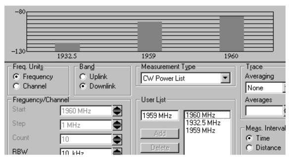
Agilent E7477A cdma2000 CW Power Measurement Display
