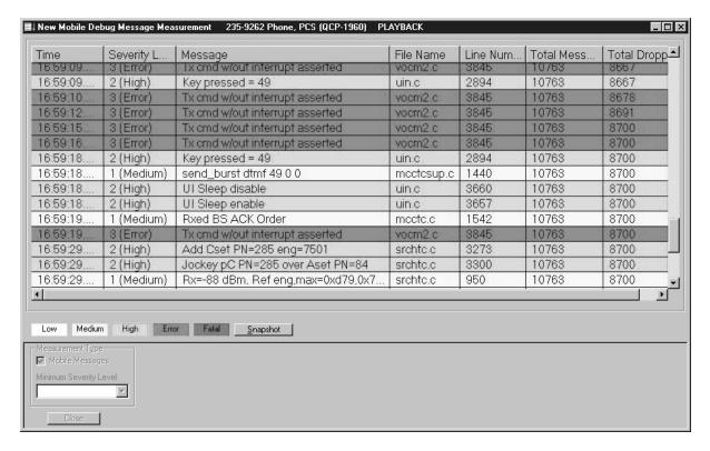
Agilent E7477A mobile debug measurement display
