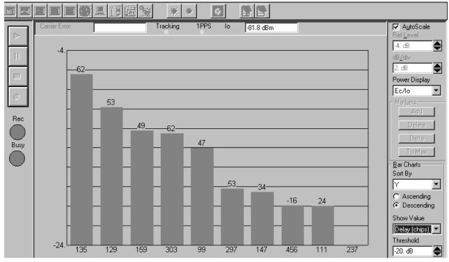
Use the timing delay measurement to troubleshoot island cell conditions
